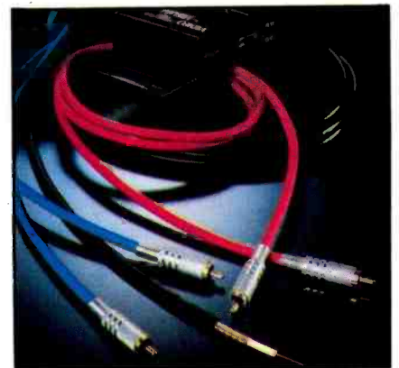
Because Osae Kamada, Hitachi chief engineer, theorized that the number of crystal boundaries in copper cable correlated to imperfect sound reproduction, linear-crystal/oxygen-free audio-visual cable has been introduced.
